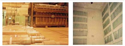
Left: Tilt-top furnace, control panel, and new custom built radiant tube burner units. Right: Old electric heat elements.
