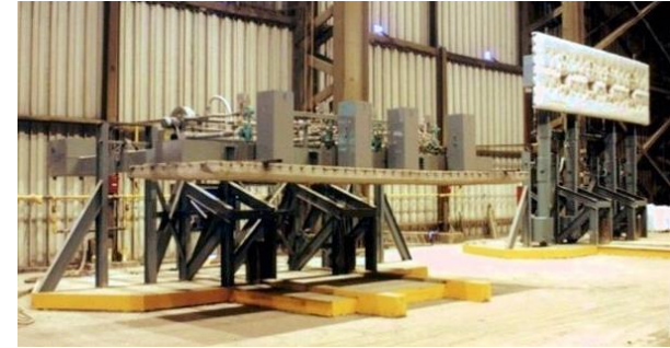
Tundish Dryers/ Dryer-Preheaters/ Preheaters
